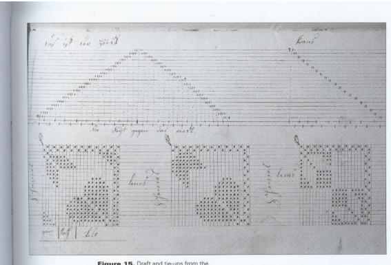
Figure 15. Draft and tie-ups from the manuscript of Jacob Schmidt. Reproduced with permission, from a private collection. This page is devoted to uneven-tied overshot designs. Note the upside-down tie-ups in relation to the threading draft.
